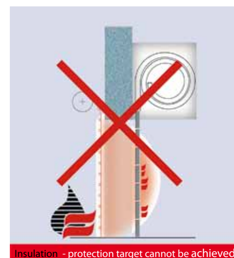
Insulation - protection target cannot be achieved
